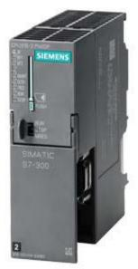
SIMATIC S7-300 CPU 315-2 PN/DP, Central processing unit with 384 KB work memory, 1st interface MPI/DP 12 Mbit/s, 2nd interface Ethernet PROFINET, with 2-port switch, Micro Memory Card required
